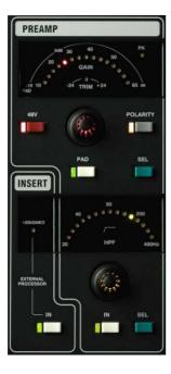
Note: To select phantom power using the processing block 48V key hold it down for 0.5 second. This is to protect against accidental operation. Red PP LEDs light on the iLive MIC/LINE input modules when phantom power is detected on their sockets, whether from their own mic preamp or an external sources. These are not available on the T Series.
